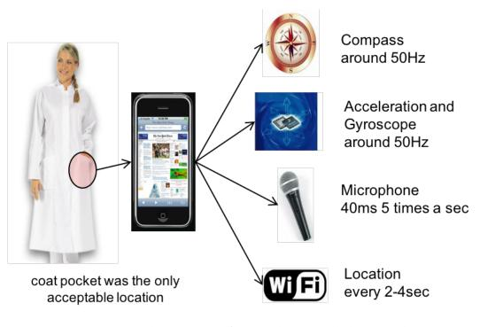
FIGURE 9.1: The position of smartphones and the available sensors.
