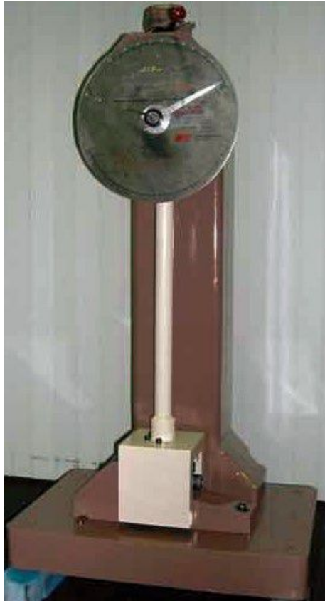
Fig. 2.4. SATEC SI-1C universal pendulum-impact testing machine [16].
