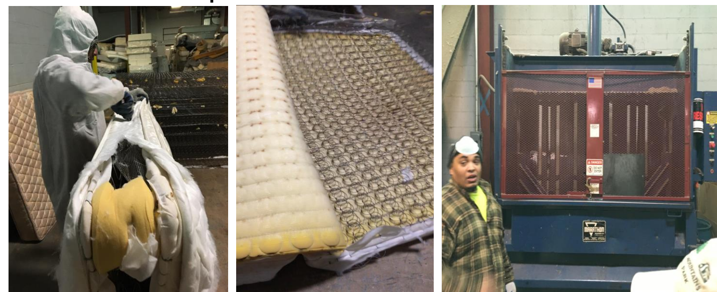
Exhibit 2. Dismantling process of an EOL mattress and vertical baler in PCG
