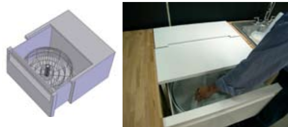
Fig. 10e Dishwasher: a 19" tall x 30" wide under counter pullout drawer, with lazy Susan style turntable dish rack and counter level hide-away lid. All dishes are accessible through the top lid or the drawer can be pulled out a few inches to gain further access.
