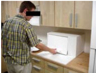
Fig. 10d Microwave: a slide-in unit into the counter surface where the turntable is at counter line enabling arthritic hands to slide hot dishes and liquids safely from within the microwave to the counter surface.
