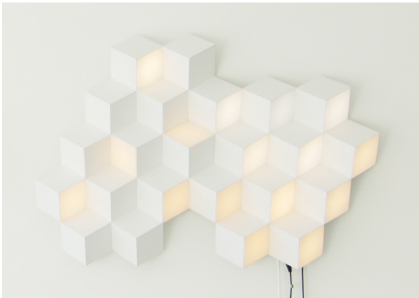
Figure 8. Integrated daylighting and artificial lighting. A close look at a section of the instrument where some surfaces is lit by daylight, some by the embedded LED. The surfaces appear in a range of lit, reflected and shadowed showing the range of local light variations. On Fig. 9 the same section is shown with the curtains drawn for the window, excluding the daylight.
