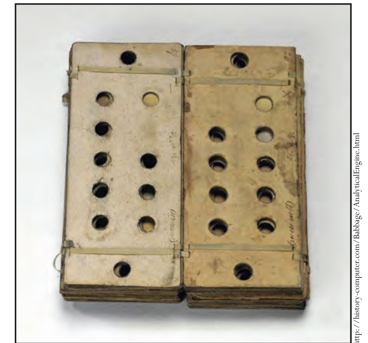
Punch cards created by Babbage to program the Analytical Machine.
