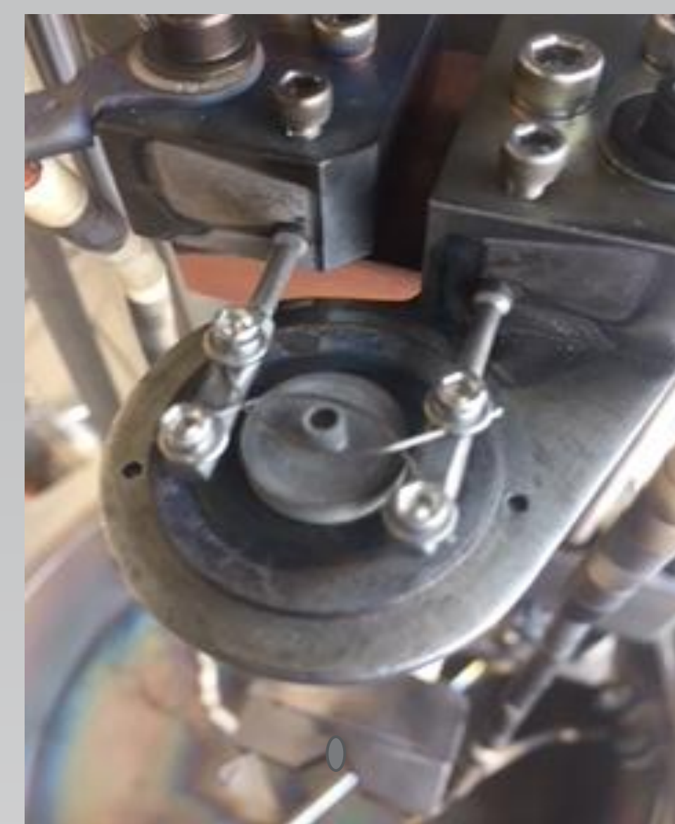
Figure 3. Tungsten filaments that are going around the molybdenum shield. A tungsten rod would go through the middle of the shield. This is only half of the pillbox, missing is the pillbox ring, pillbox top, and upper insert.
