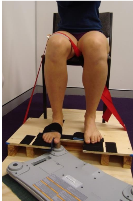
Figure 5-1 Experimental set up for strength testing of the flexor hallucis muscle of the right foot.
