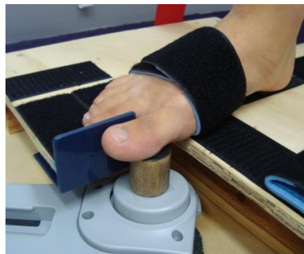
Figure 5-2 Close up image of the position of the foot on the platform The foot is secured with Velcro and the position of the sensor placed under the interphalangeal joint of the big toe.
