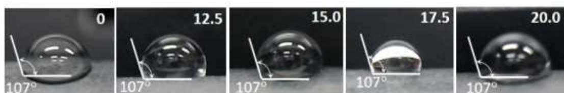
Fig. 5 – Contact angle measurements on the carbonised sugar membrane surface (permeate side) as a function of NaCl concentration from 0 to 20 wt%.
