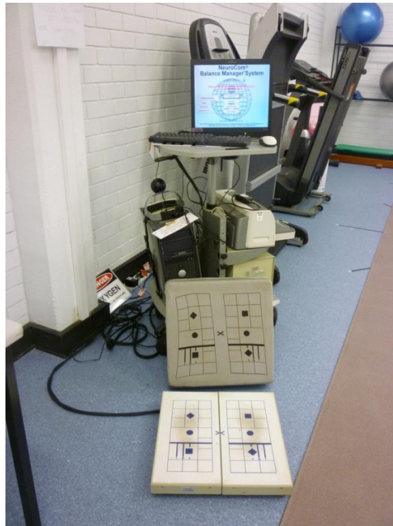
Figure 3.1 Image of the Basic Balance Master system. The foam cushion provided with the equipment is shown propped up behind the firm surface force plate.
