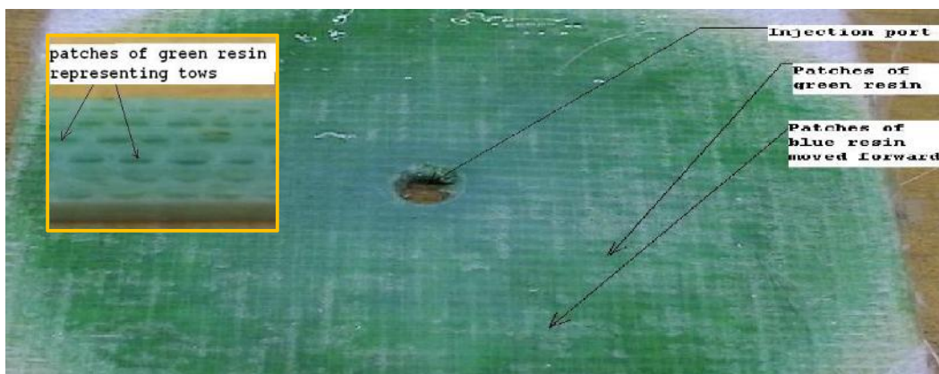
Figure 2.43 Two-colour experiment [217]: specimen and micrograph of the cross section
