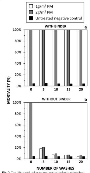
**Fig. 2** The efficacy of polyester netting treated with pirimiphosmethyl (PM) against pyrethroid-susceptible insectary-reared *Anopheles gambiae* in terms of mosquito mortality as measured with standardized wire ball assays with and without the binder
