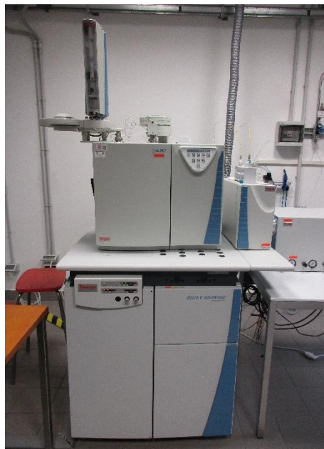
Fig. 5.1 The Thermo Scientific Delta V Advantage Isotope Ratio Mass Spectrometer present at the Geosciences Department, University of Padova.
