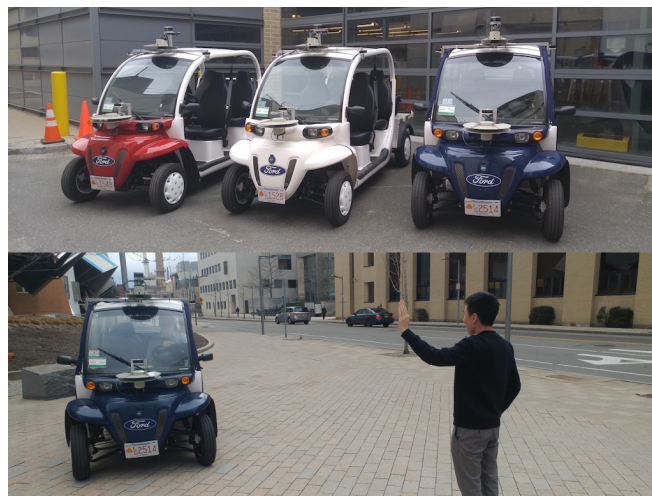
Fig. 1: A fleet of three electric shuttles operates on MIT campus. The shuttles are manually driven but equipped with camera and Lidar for sensing pedestrians. Customers may hail rides directly from any nearby shuttle.
