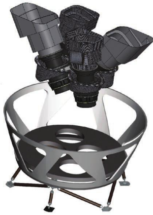
Figure 5. Left. —Diagram illustrating the orientations of the four TESS cameras, lens hoods, and mounting platform. Right. —Artist's conception of the TESS spacecraft and payload.
