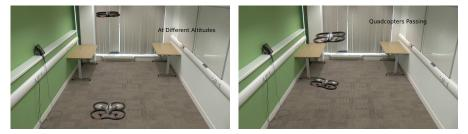
(c) UAVs manage to coordinate, one fly in high (d) UAVs are flying in different directions, sucand the other in low altitude. cessfully passing.
