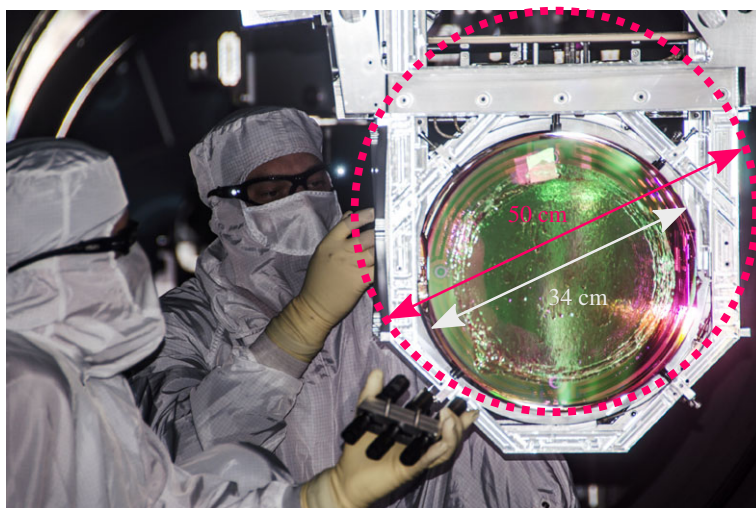
Figure 2. An aLIGO test-mass mirror 34 cm in diameter. (Photo: www.ligo.org .) The pink dotted circle indicates the proposed size of a mirror for the Einstein Telescope with a diameter of 50 cm. (Note that the mirror surface in the photo is covered by a protective film which makes it look rough.)
