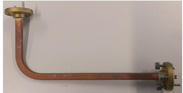
Fig. 4 A photo of a smoothly curved waveguide bend made for test.
