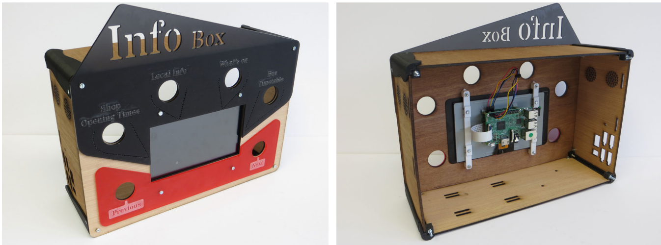
Figure 3. Example of the Inventor Kit used to build the Info Box prototype, before addition of buttons.
