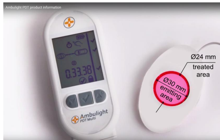
Figure 4.1: Ambulight PDT device. The emitting head has a diameter of 30 mm but the treated area can be up to 24 mm to prevent any marginal failure due to misalignment of the area or intensity drop at the edges. The battery pack shows information on the display about remaining time and the treatment mode. The pictures were taken from Ambulight PDT product information video.
