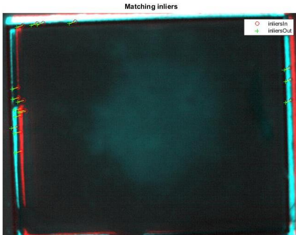
Figure 2 RANSAC geometrical transformation – the blue and the red contours are the fluorescent reference contours of the first and the second images correspondingly. The inliers and the outliers are the corresponding points which allow the rotation and the positioning of the second image with the regard to the first image.
