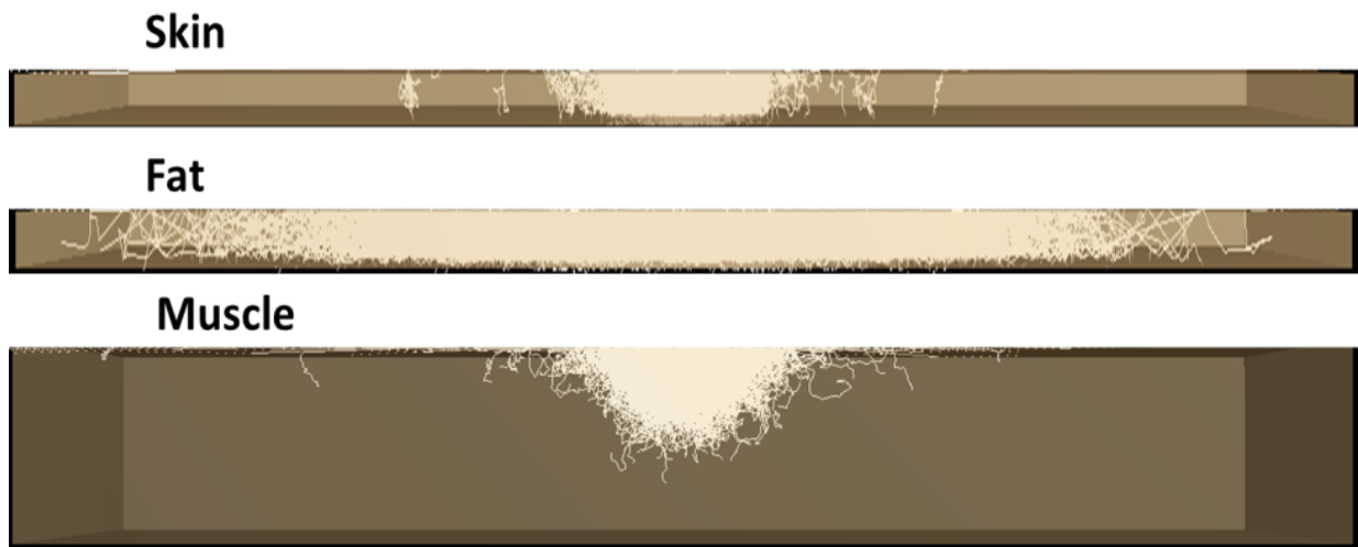
Figure 6.6: Light propagation from the OLED made from Super Yellow polymer in individual layers of 2 mm thick skin, 2 mm thick adipose fatty tissue and 30 mm thick muscle.
