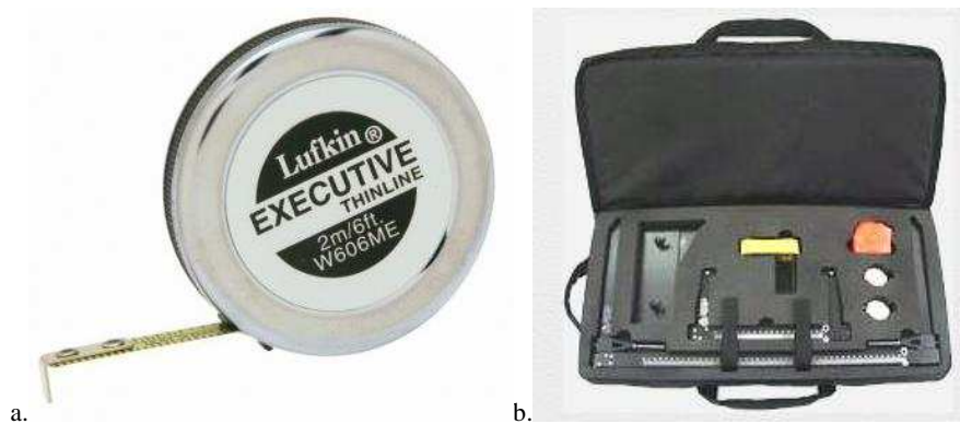
Figure 2.1: a) Anthropometric tape measure (Lufkin, 2016) and b) Rosscraft Centurion anthropometry kit (Rosscraft, 2016).
