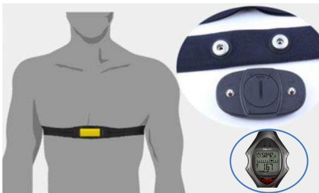
Figure 3.3. Left: The position of a polar heart rate monitor strip for recording heart rate. Top right: a close-up of the heart rate sensor. Bottom right: the Polar watch.
