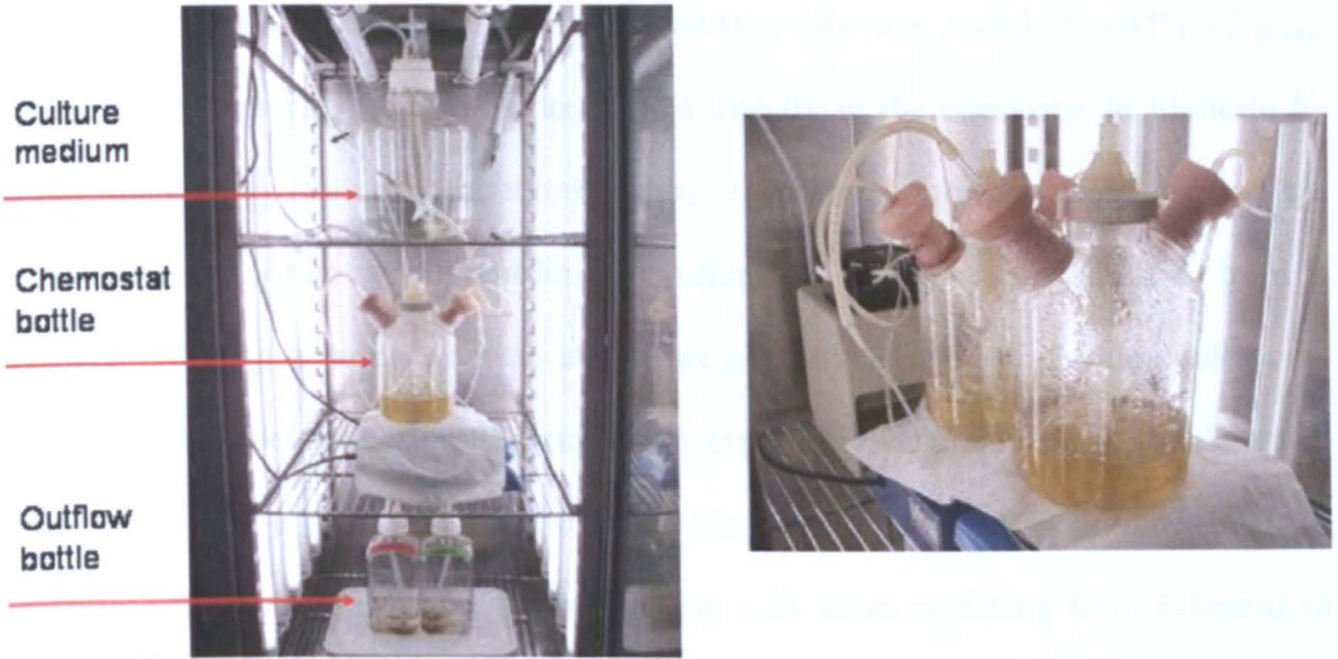
Figure 5-1: On the left, the entire chemostat set-up in the culture chamber with the culture medium bottle on the top, the chemostat bottle on the middle, and the outflow bottle on the bottom shelf. On the right, a close-up of the chemostat bottle with inflowing medium, effluent culture and bubbling. Photos are courtesy of François Ribalet.
