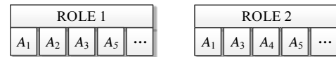
Fig. 1. Difference of access rights between two different roles in the traditional RBAC model
