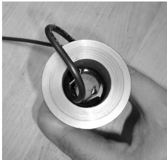
Figure 6 – Geophone potted in push cone cavity
