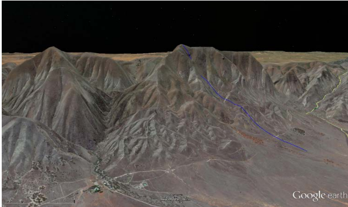
Figure 2: Synthetic Google Earth image (vertical scale exaggerated) of hills east of Spencer Gulf (South Australia) with up to 600m head showing a hypothetical off-river PHEs system (blue line)
