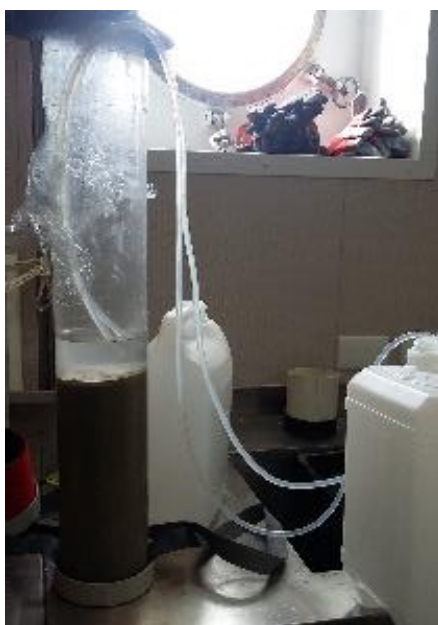
Figure 59. Example of bottom water sampling from Multicore.
