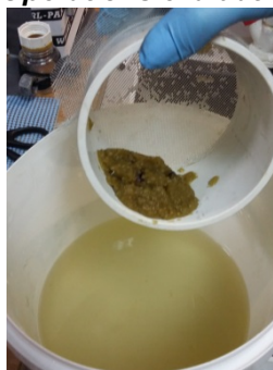
Figure 71. Re-sieving of 100µm plankton net sample.
