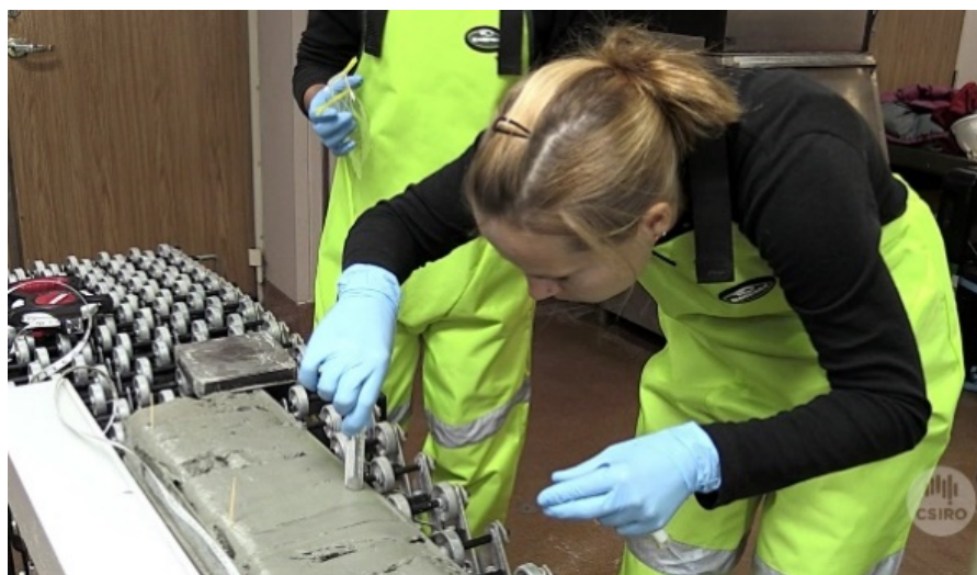
Figure 58. aDNA sampling from Kasten Core using minicores.
