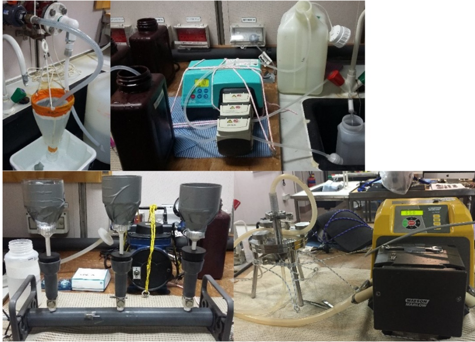
Figure 74. Underway seawater lab sampling set-up. From top left to bottom right: 25 µm plankton net; 3-head Watson and Marlow peristaltic pump used for DNA, HBI filtration; vacuum pump for Chlorophyll, phytoplankton; Watson and Marlow peristaltic pump with a 142mm filter holder.
