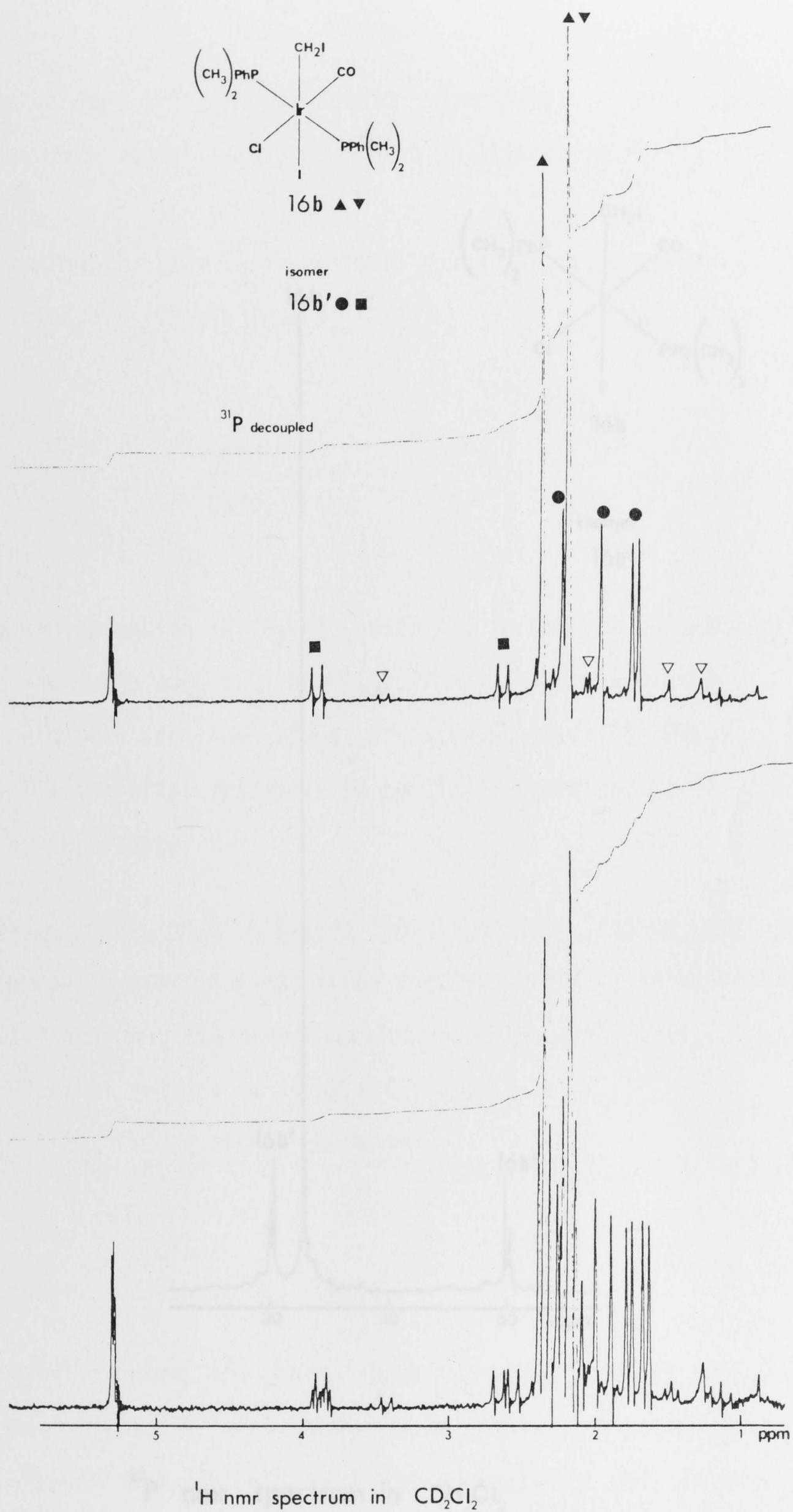
Figure 8. 1 H NMR Spectrum of Product from Reaction of CH 2 I 2 with IrCl(CO)(PPhMe 2 ) 2 . ▲ PCH 3 of 16b; ▼ IrCH 2 I of 16b; ● PCH 3 of 16b'; ■ IrCH 2 I of 16b'; ▽ impurities.
