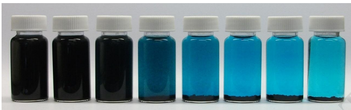
Figure 4: Suspensions of SDS exfoliated graphene with 10 ppm methylene blue 10, 30, 60 min, 120, 240, 480, 1140 and 2880 min after initial contact with dye at 25 °C.
