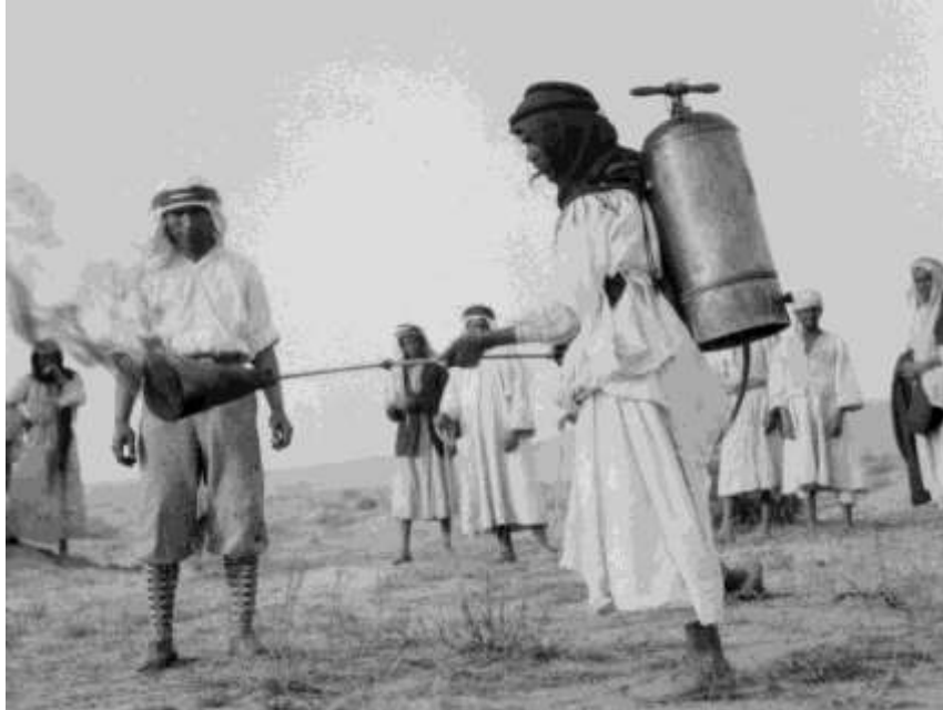
Figure 8.3. Flame gun for locust control being tested in Palestine, 1915. Similar designs were still used in Egypt during the 1930s (photo courtesy Keith Cressman, FAO). 24
