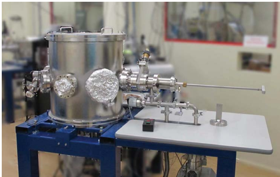
Figure C.20: Chamber and loadlock mechanism on the new ERD/RBS line, attached to second line of NEC 5SHD accelerator.
