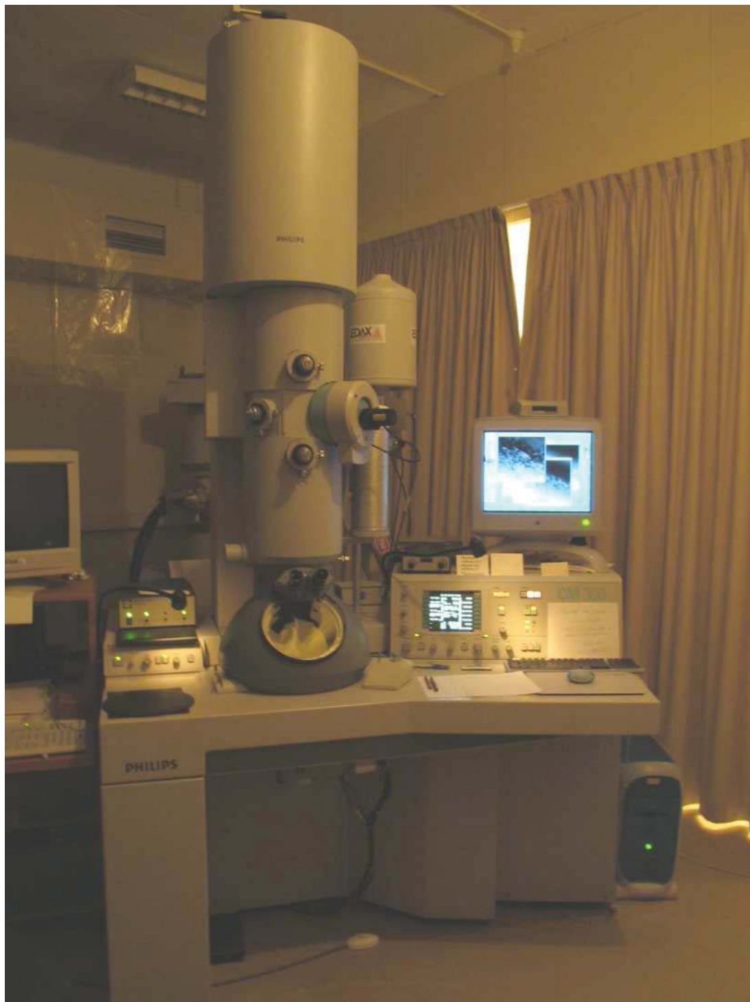
Figure B.9: The Philips CM300 transmission electron microscope located in RSES, ANU, used for all TEM analysis in this study.
