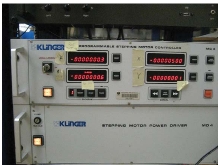
Figure C.4: Relative encoder and stepping motor operating the new RBS/ERD line's goniometer. Readouts show (clockwise from top left) the rotation \alpha , translation x , translation y and tilt \beta of the goniometer and hence sample stage. Beneath the readouts are manual operating controls, when the system is not slaved to the software (i.e., software inactive).
