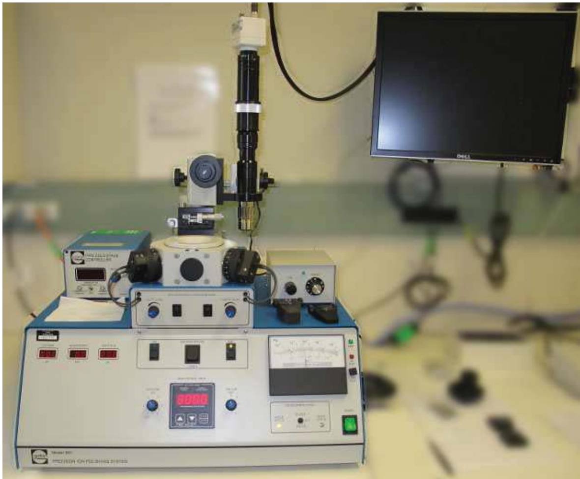
Figure B.12: Gatan Precision Ion Polishing System (PIPS) ion mill. After TEM samples have reached thicknesses of \sim 5 \mu\text{m} in the region of interest, electron transparency is produced by milling with Ar ions at energies up to 6 keV under vacuum upon a rotating stage.
