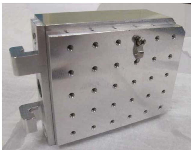
Figure C.21: Specialised mounting puck designed for the new ERD/RBS line goniometer system.
