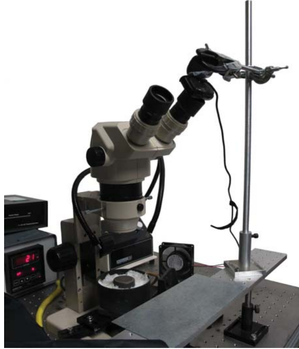
Figure 3.9: Apparatus designed to observe hydrogen blisters and craters forming during the annealing process.
