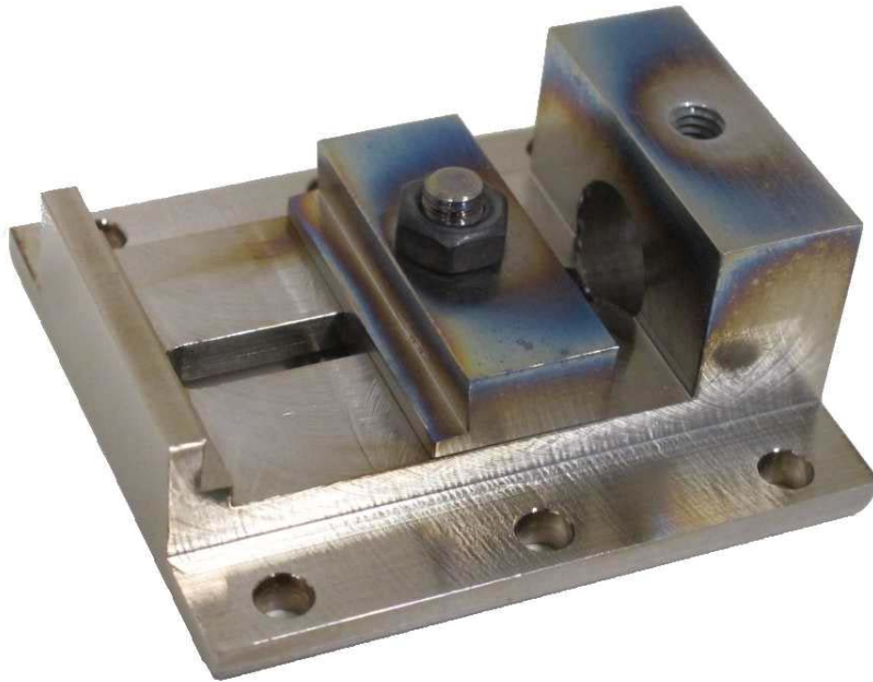
Figure B.16: Photograph of stress boat apparatus with the originally designed small shelves mounted, as discussed in Section 3.3.2.
