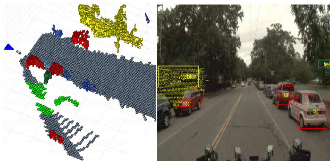
Figure 2.17: Semantic representation of one of the labeled scenes. Left image: 3D view of the inferred class labels. The blue triangle indicates the vehicle’s position. Right image: The inferred labels as well as the ROIs and the projected laser returns. The color of each ROI matches the color of the associated object in the 3D plot [29].
