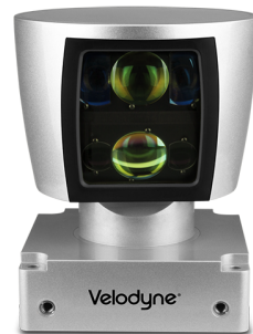
Figure 2.8: Velodyne 64E with rotating beam and 64 laser rays
