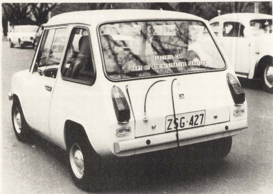
PLATE 11.1 The Enfield 8000 — showing its plug-in recharging connection. Electric Commuting Car No. 859 off the production line at the Enfield Works in England. It weighs one tonne with half the weight in its eight 12-volt batteries (the engine is only a tenth of the weight of the batteries and hidden away behind the seats). It recharges overnight from a 240 volt supply and has a range the next day of 50 kilometres. (Canberra Times, 14 September 1977)
