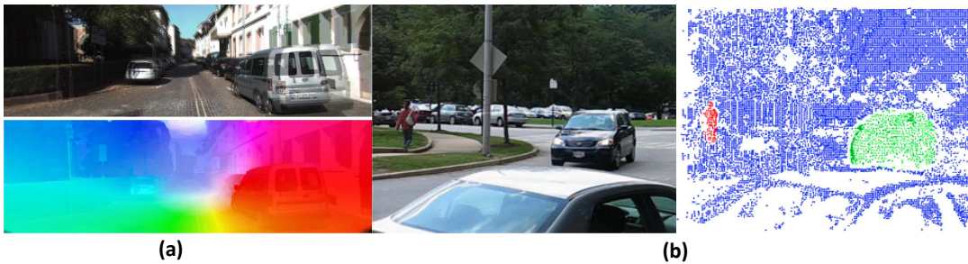
Figure 1.3: (a) A sample result of optical flow from [Yang and Li, 2015]. Top: overlay of two input frames. Bottom: estimated flow (overlayed onto the original image); (b) An example of motion segmentation [Brox and Malik, 2010]. Only motion information was used to successfully separate the car (green) and even the pedestrian (red) from the background.
