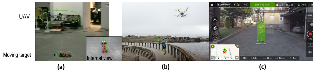
Figure 1.1: Tracking algorithms can be used to send visual information for controlling drones. (a) A color histogram based drone tracking system [TeuliÁlre et al., 2011]; (b) In a real-life scenario, the DJI Phantom 4 uses ActiveTrack technology to track moving subjects and avoid obstacles automatically. (c) A screen capture of the Graphical User Interface (GUI) of the Phantom 4. The person over-shaded by green is the target.
