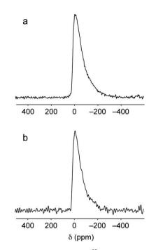
Fig. 4  $^{25}$ Mg (20.0 T) MAS NMR spectra of (a)  $^{25}$ Mg-enriched anhydrous wadsleyite and (b) wads-H. Spectra are the result of coadding (a) 109 552 and (b) 163 840 transients separated by a recycle interval of 0.5 s. For wads-H an initial DFS pulse was used to increase signal sensitivity. In both cases the MAS rate was 30 kHz.
