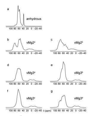
**Fig. 3** Simulated <sup>17</sup>O (20.0 T) MAS NMR spectra for (a) anhydrous wadsleyite and (b–g) fully hydrated ordered model structures for hydrous wadsleyite based on calculated NMR parameters. Lorentzian line broadening factors of (a) 200 Hz and (b–g) 400 Hz were applied prior to Fourier transformation of the simulated FIDs.
