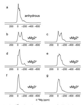
**Fig. 5** Simulated <sup>25</sup>Mg (20.0 T) MAS NMR spectra for (a) anhydrous wadsleyite and (b–g) fully hydrated ordered model structures for hydrous wadsleyite based on calculated NMR parameters. In each case a Lorentzian line broadening factor of 400 Hz was applied prior to Fourier transformation of the simulated FID.
