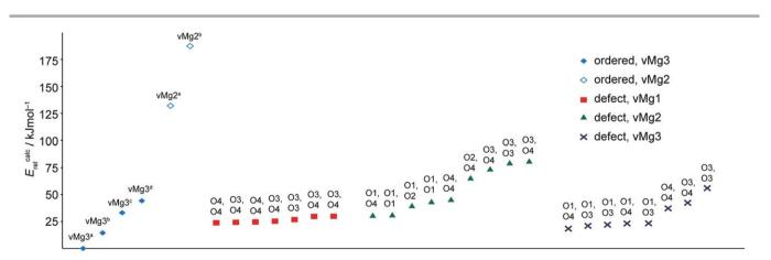
**Fig. 9** Calculated total energies for fully hydrated ordered model structures (represented by empty and filled blue diamonds) and structures containing a hydrated defect at an alternative cation site (represented by squares, triangles and crosses). For the defect model structures, the oxygen sites to which the hydrogen atoms are bonded within the alternative defect are indicated. Energies are shown relative to the lowest energy structure, vMg3<sup>a</sup>.
