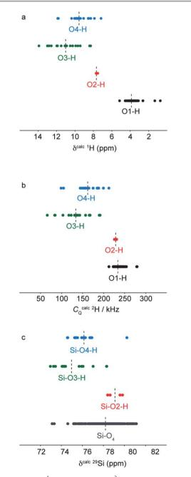
**Fig. 10** Calculated (a) <sup>1</sup>H chemical shifts, (b) <sup>2</sup>H quadrupolar coupling and (c) <sup>29</sup>Si chemical shifts for all H and Si sites in the ordered and defect-containing model structures, grouped by local bonding environment. Average values for each group of parameters are indicated by dashed lines.
