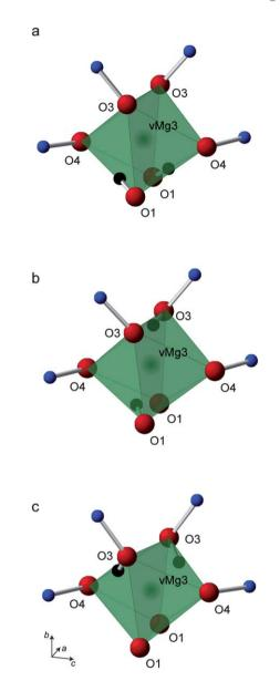
**Fig. 12** Expanded views of proposed models for hydrated defects surrounding the vacant Mg3 octahedron (shown in green) in the structure of hydrous wadsleyite. Vacancies are shown containing (a) two hydroxyl, (b) one hydroxyl and one silanol, and (c) two silanol protons. Oxygen, silicon and hydrogen atoms are represented by red, blue and black spheres, respectively. The nomenclature of the oxygen species is as given in the anhydrous crystal structure.<sup>10</sup>
