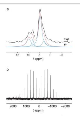
**Fig. 7** (a) Rotor-synchronised and (b) wide-spectral width <sup>2</sup>H (14.1 T) MAS NMR spectra of wads-D. A deconvolution of the experimental spectrum in (a) is shown below the MAS lineshape in red, with individual components shown in blue. Spectra are the result of coadding (a) 4126 and (b) 12 378 transients separated by recycle intervals of 5 s. MAS rates were (a) 12.5 kHz and (b) 20 kHz.
