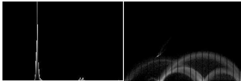
Figure 2. On the left is an value (1D) histogram and on the right is the value-gradient magnitude (2D) histogram of tooth dataset [25]. In both the graphs, value is plotted along the horizontal axis. The gradient magnitude is along the vertical axis in the 2D histogram.
