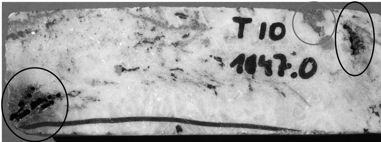
Figure 4. Drill core sample T-10, at 1047 m, shows carbonatite vein material with pyrrhotite. Fine-grained pyrrhotite masses selected for Re-Os dating are shown within black circles. A pyrrhotite patch with a thin pyrrhotite rim around a pyrrhotite core is circled in gray. Length of core is 10 cm. A color version of this figure is available in the online edition or from the Journal of Geology office.
