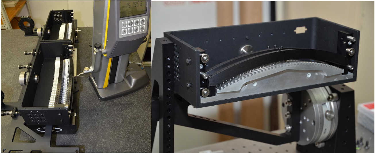
Figure 15. The two curved slit assemblies on the translation stage, right: single V-groove block for lens mounting 40 lens sets
