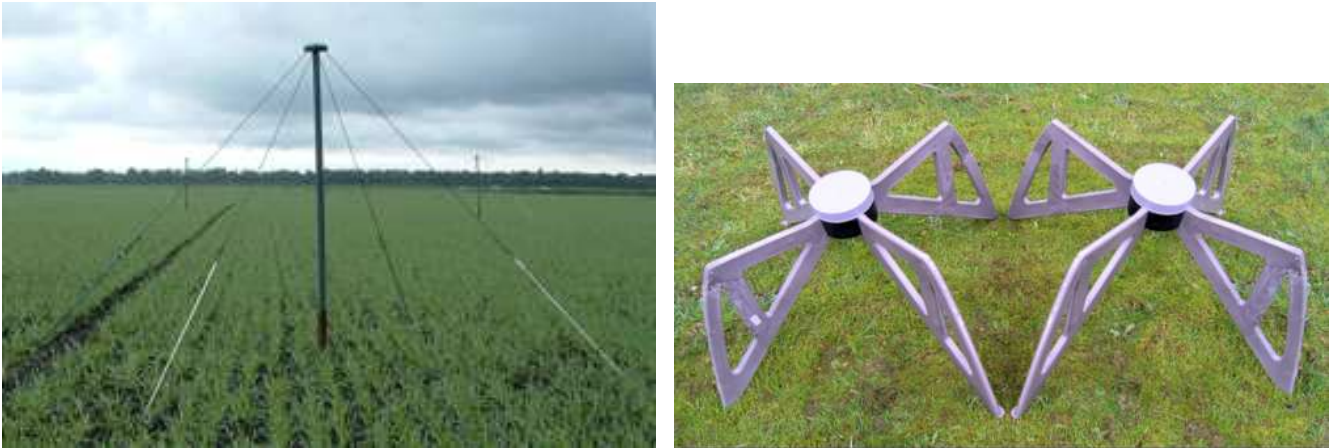
Fig. 1. Pictures of prototypes of the LOFAR antennas. ( left ) The low-frequency antenna, optimised for the 30–80 MHz frequency range. ( right ) The high-frequency antenna, optimised for the 115 - 240 MHz range.
