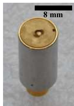
Figure 9. 6 The photograph of the imperfect curve within the active area of a focused PZT transducer.
