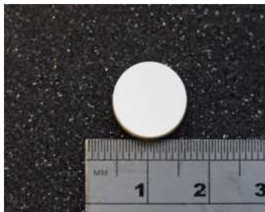
Figure 6.16 Green 50BCZT gel cast sample obtained from 45 vol% solids loading with 30wt% resin and 2.4 wt% Dispex AA4040 after demoulding.
