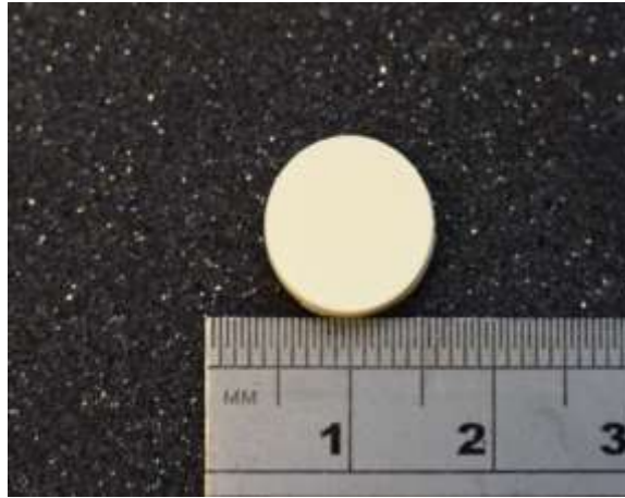
Figure 7.9 Green PZT gel cast sample obtained from 48 vol% solids loading with 20wt% resin and 1 wt% Dispex AA4040 after demoulding and drying.
