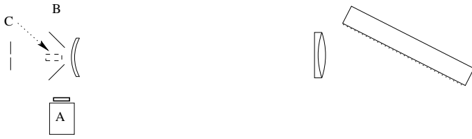
Fig. 1. Schematic view of the TRIPPEL spectrograph as seen from above. Components from left to right: entrance slit, pick-off mirrors for ports A-C, field lens, Littrow doublet, grating. Spectral port A has a CCD camera with an interference filter.
