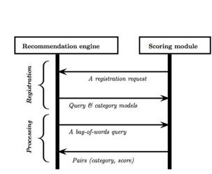
The phases of interaction between the recommendation engine and a scoring module of the architecture presented in Figure 1.
