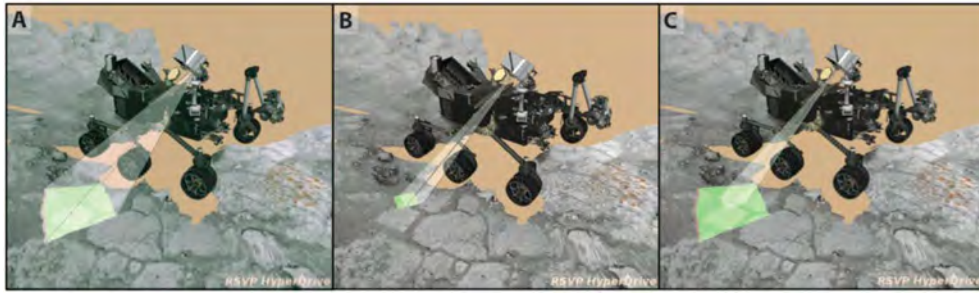
Figure 2. RSVP hyperdrive modeling of clast survey image positions. (a) Position of M-34 image footprint. (b) Position of M-100 image footprint. (c) Combined M-34 and M-100 image footprints. Differences in sighting between M-34 and M-100 images, combined with the angle of viewing for the clast survey results in location of the M-100 image frame near the lower right-hand side of the M-100 image frame.
