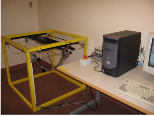
Fig. 1. Experimental setup. A laboratory-scale 3-D crane system.
