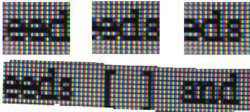
Figure.5 – Stitching of multiple images using Stick-on mobile microscope. Around ten individual microscope images (top- 3 representative images) are sequentially stitched along linear to form a large image mosaic (bottom).
