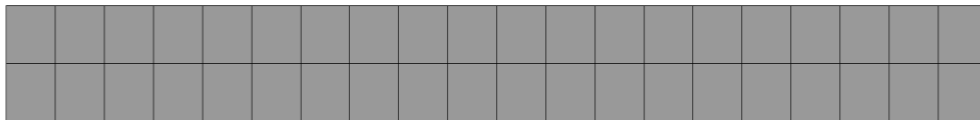
Figure 8.12 Element mesh used for modeling the bimorph piezoelectric beam in HFS-FEM analysis.
