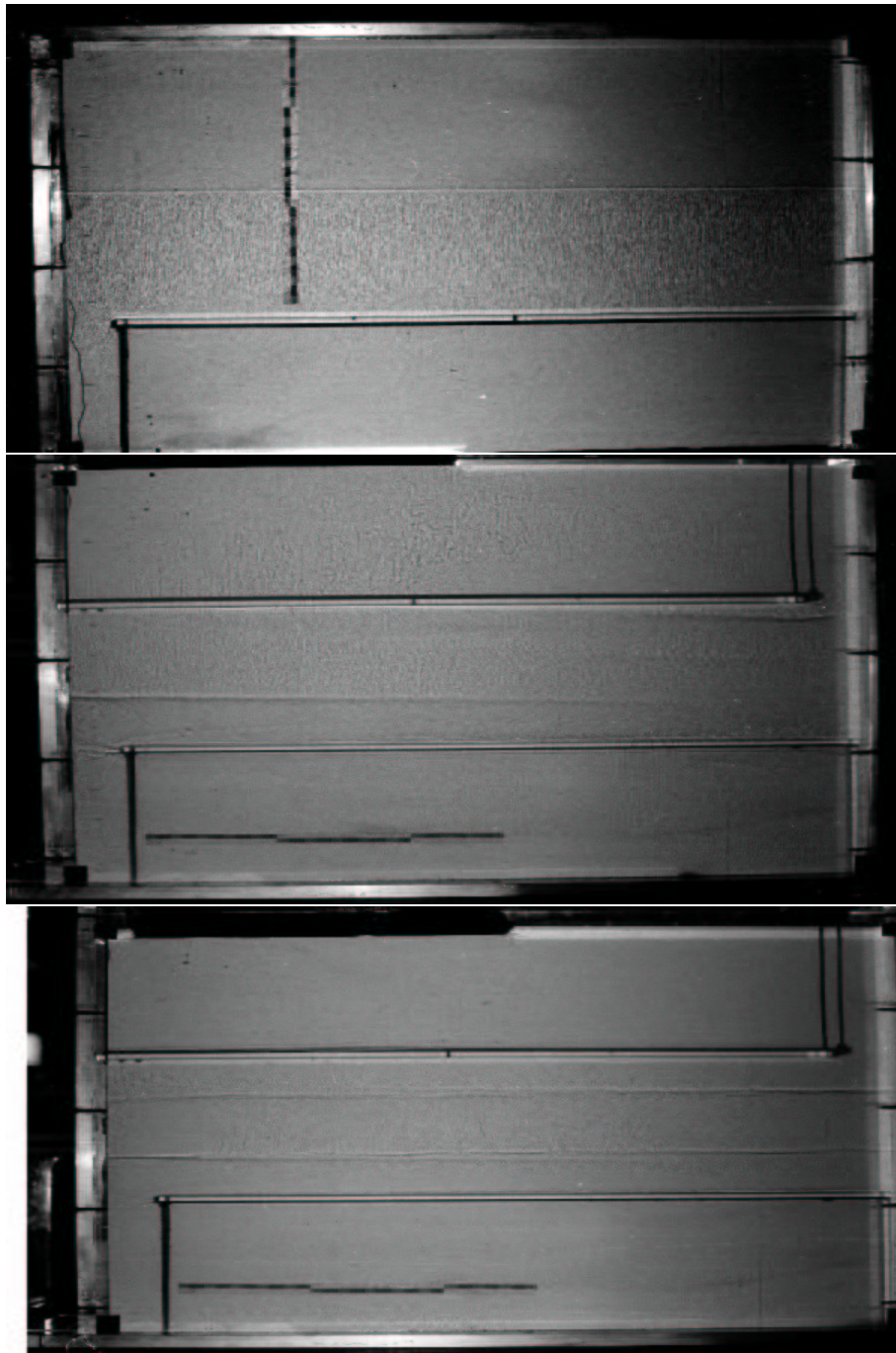
Figure 4.9: Three successive shadowgraphs of the cross gradient experiments by Turner (1974). In the first photograph, only the bottom salt reservoir and the middle salt finger region are in place. When the top sugar reservoir was added, the shearing set up by the horizontal differences in vertical buoyancy flux led to bands in the shadowgraph. The third photograph shows the subsequent breakdown into a series of convecting layers.
