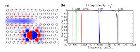
Fig. 3. Double-defect waveguide-cavity structure with the cavity created by two defect rods with the radius  $r_{def}$ : (a) Electric field at the resonance reflection for  $r_{def} = 0.121a$ ; (b) Transmission spectra for different values of  $r_{def}$ : 0.119*a* (black), 0.120*a* (blue), 0.121*a* (red), 0.1213*a* (green).
