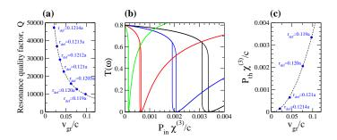
Fig. 4. (a) Quality factor Q vs. group velocity  $v_g$  at resonance for the structure shown in Fig. 3; (b) Nonlinear bistable transmission in the same structure at the frequencies with 80% of linear light transmission vs. the incoming light power for different values of  $r_{def}$ : 0.119*a* (black), 0.120*a* (blue), 0.121*a* (red), 0.1214*a* (green); (c) Switch-off bistability threshold  $P_{th}$  vs. the group velocity  $v_g$  at resonance for the same structure.
