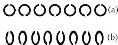
FIG. 1. Schematic of a one-dimensional array of split-ring resonators in (a) planar and (b) axial geometries. The axes of the split-ring resonators as well as the magnetic component of the applied field are directed in parallel. The electric field component is transversal to the slits.
