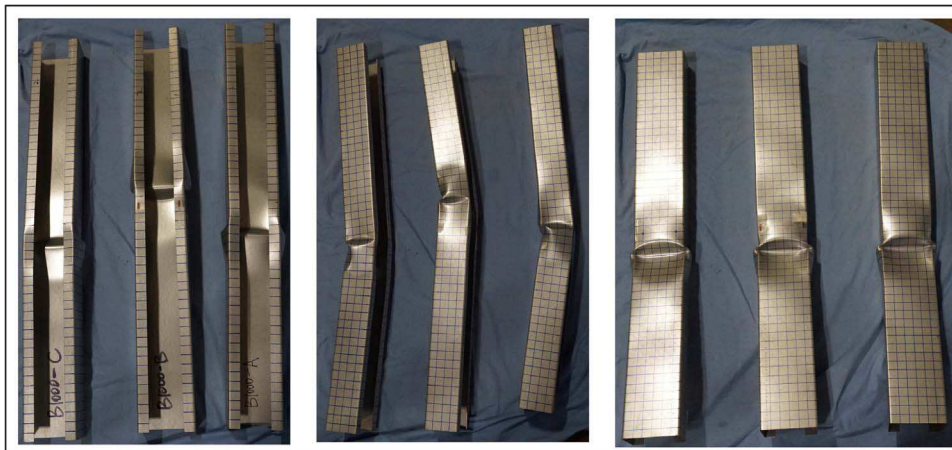
Fig. 12. Failure modes of 1 m long columns with type B cross-section.
